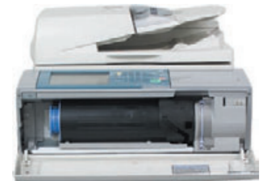
The long-life black toner can even be changed during operation.
